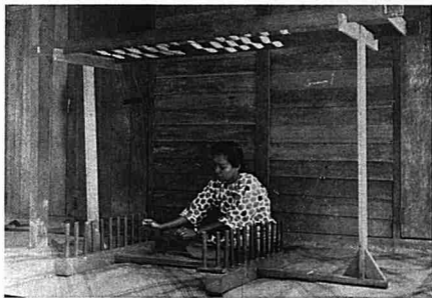
A pengani fixing the chorak by arranging on the anjan the warp threads selected from the loaded spools on the metak above it.
