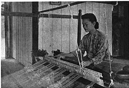
Close-up of the karap assembly. A belira bunga is inserted to separate component sections of the warp for weaving a kain songket .
